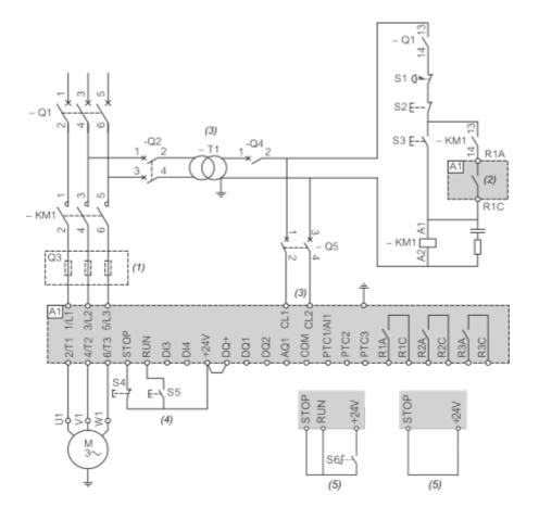
Connection in line, with line contactor, no bypass, type 1 or 2 coordination, non - reversing, 2-wire or 3-wire control
